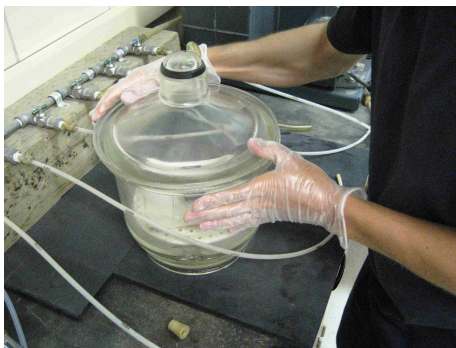
Figure 3.6: Picture of elastomer specimen in vacuum chamber
