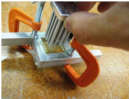
Figure 3.9: Picture of placing heat sink into epoxy mold
